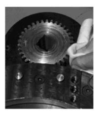
Fig. 24 Drive gear of the gear ring
