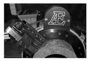
Fig. 11 Attaching the tool slide
