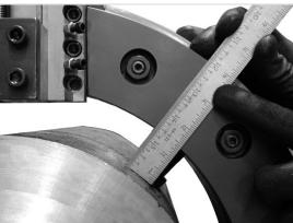
Fig. 12 Aligning the split frame
