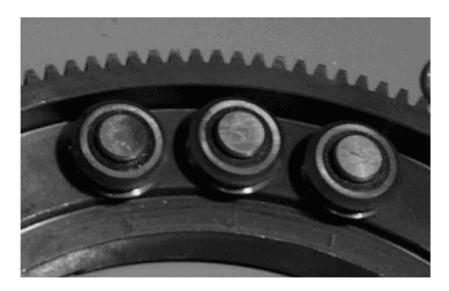
Fig. 26 Split frame bearings
