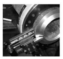
Fig. 20 Pipe beveling completed
