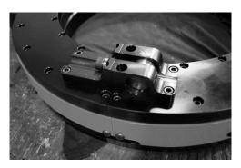
Fig. 10 Aluminum split frame showing different swing bolt arrangement
